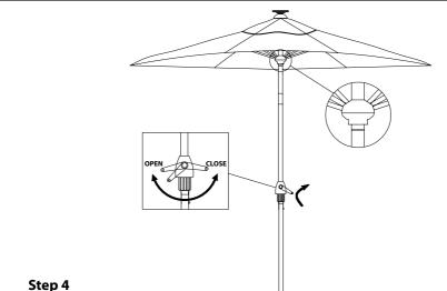
Keep turning the crank to tilt the parasol after it is fully open.
